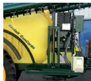
Cleaning system Automatic cleaning system with a separate cleaning tank, secures both a clean system, and no mix of different chemicals
