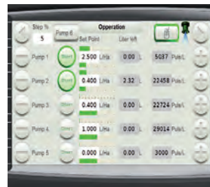
Operating The dosage and the mix of chemicals is controlled from the drivers cabin.
